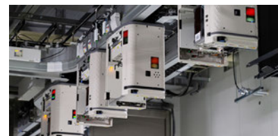
Transportation equipment inside the clean room
