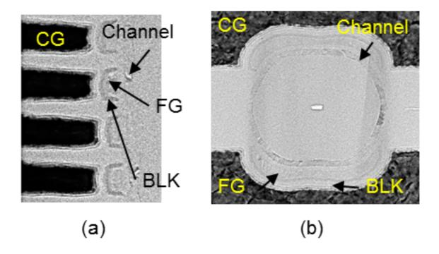
Figure 1- Fabricated semicircular FG cells (a) Cross-sectional view (b) Plane view
