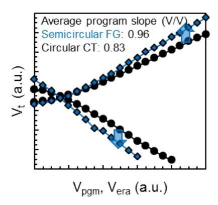
Figure 2 - Experimental program/erase characteristics comparing the semicircular FG cells with the circular CT cells
