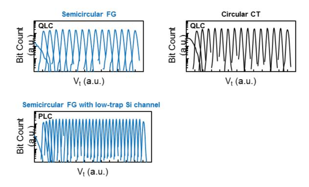
Figure 3. Simulated Vt distributions after programming using calibrated parameters
