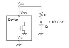
This data may vary from device to device. We recommend to use this data as a reference for selecting a resistor value.
