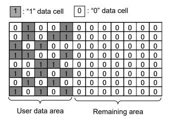
(a) Accelerate block endurance degradation by fixed dummy "0" data write User data area
