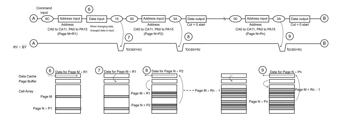
6. Address for Page (M + R1) is input. If the data needs to be changed, changed data is input.
