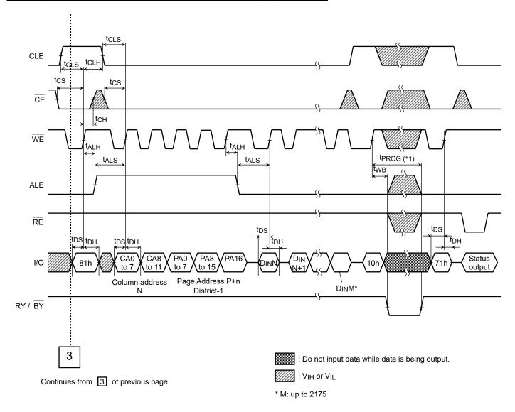
(\*1) tpROG: Since the last page's programming by 10h command is initiated after the previous cache program, the tpROG during cache programming is given by the following equation.
