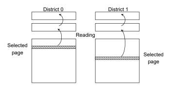
The data transfer operation from the cell array to the Data Cache via Page Buffer starts on the rising edge of WE in the 30h command input cycle (after the 2 Districts' address information has been latched).
