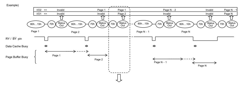
If the Page Buffer Busy returns to Ready before the next 80h command input and Status Read is done during this Ready period, the Status Read provides the Pass/Fail result for Page 2 on I/O1 and the Pass/Fail result for Page1 on I/O2.
