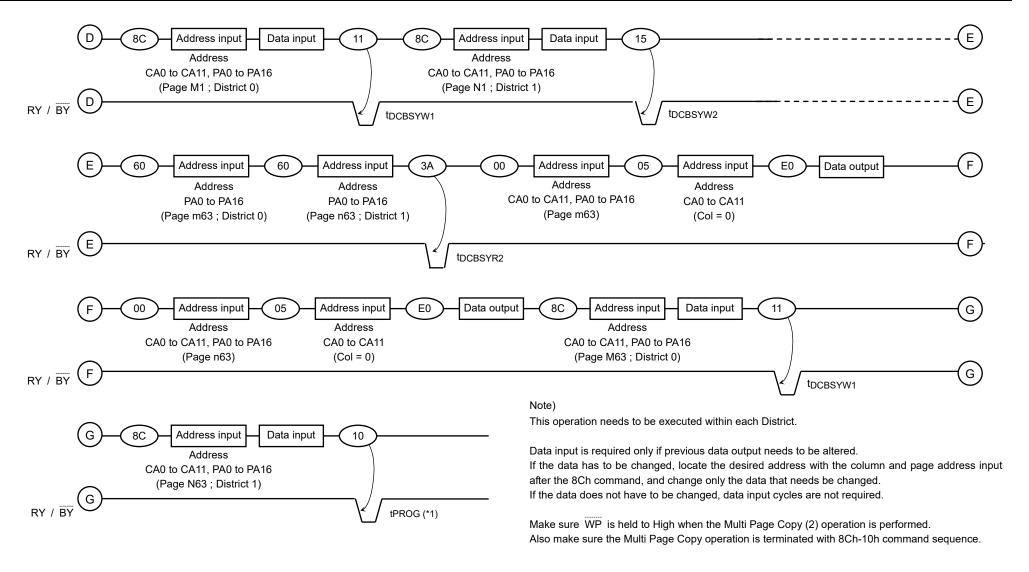
(\*1) tPROG: Since the last page's programming by 10h command is initiated after the previous cache program, the tPROG during cache programming is given by the following equation.
