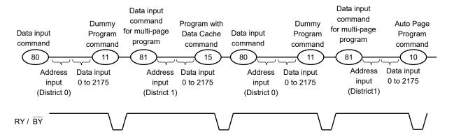
After either "15h" or "10h" Program command is input to the device, physical programing starts as follows. For details about Auto Page Program with Data Cache, refer to "Auto Page Program Operation with Data Cache".
