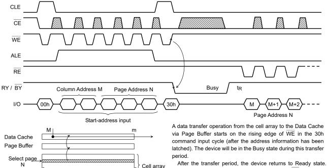
After the transfer period, the device returns to Ready state. Serial data can be output synchronously with the RE clock from the start address designated in the address input cycle.
