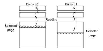
The data transfer operation from the cell array to the Data Cache via Page Buffer starts on the rising edge of WE in the 30h command input cycle (after the 2 Districts' address information has been latched).
