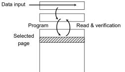
The data is transferred (programmed) from the Data Cache via the Page Buffer to the selected page on the rising edge of WE following input of the "10h" command. After programming, the programmed data is transferred back to the Page Buffer to be automatically verified by the device. If the programming does not succeed, the Program / Verify operation is repeated by the device until success is achieved or until the maximum loop number set in the device is reached.
