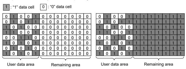
(a) Accelerate block endurance degradation by fixed dummy "0" data write
