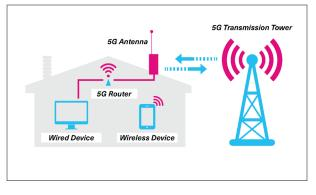
Figure 3: A 5G fixed wireless access configuration
