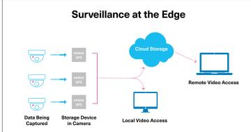
Figure 5: Enterprise security camera edge configuration
