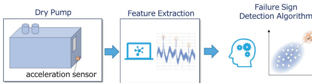
Figure 6. Failure sign detection of dry pump utilizing AI
