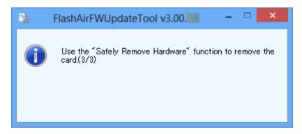
When the product is removed from a SD card slot, the following window is displayed. Insert the product again, and click the "OK" button.
