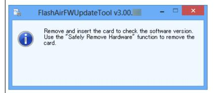
When the product is removed from a SD card slot, the following window is displayed. Insert the product again, and click the "OK" button.
