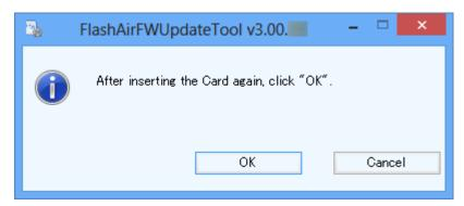
The product software update will start. While the below window is displayed, do not remove the product from the SD card slot or turn off the PC. The software update will fail, and the product may no longer start up.
