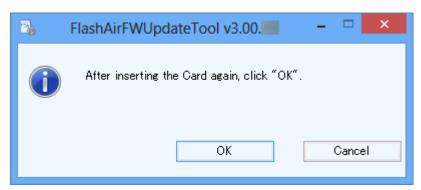
Preparations to update the product start. While the below window is displayed, do not remove the product from the SD card slot or turn off the PC. The software update will fail, and the product may no longer start up.
