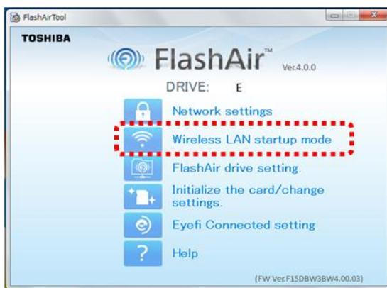
Select Automatic startup mode or Manual startup mode on FlashAir setting and click the "Apply" button.
